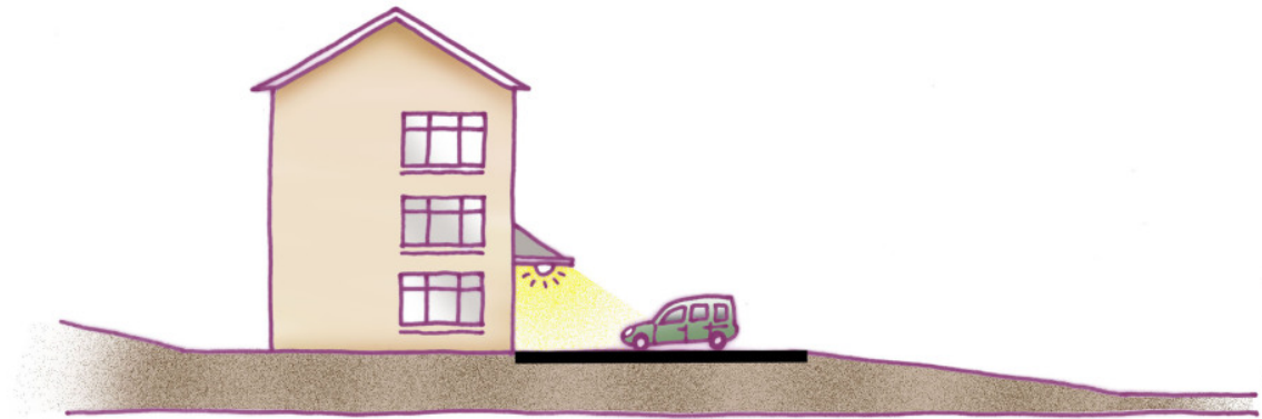
Car parking close to and with level or gently sloping approach to main entrance. Main entrance covered and lit.
